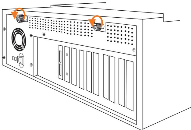
3. Remove the L shape metal bracket at rear of NA255A by loosening the screw on metal bracket.
