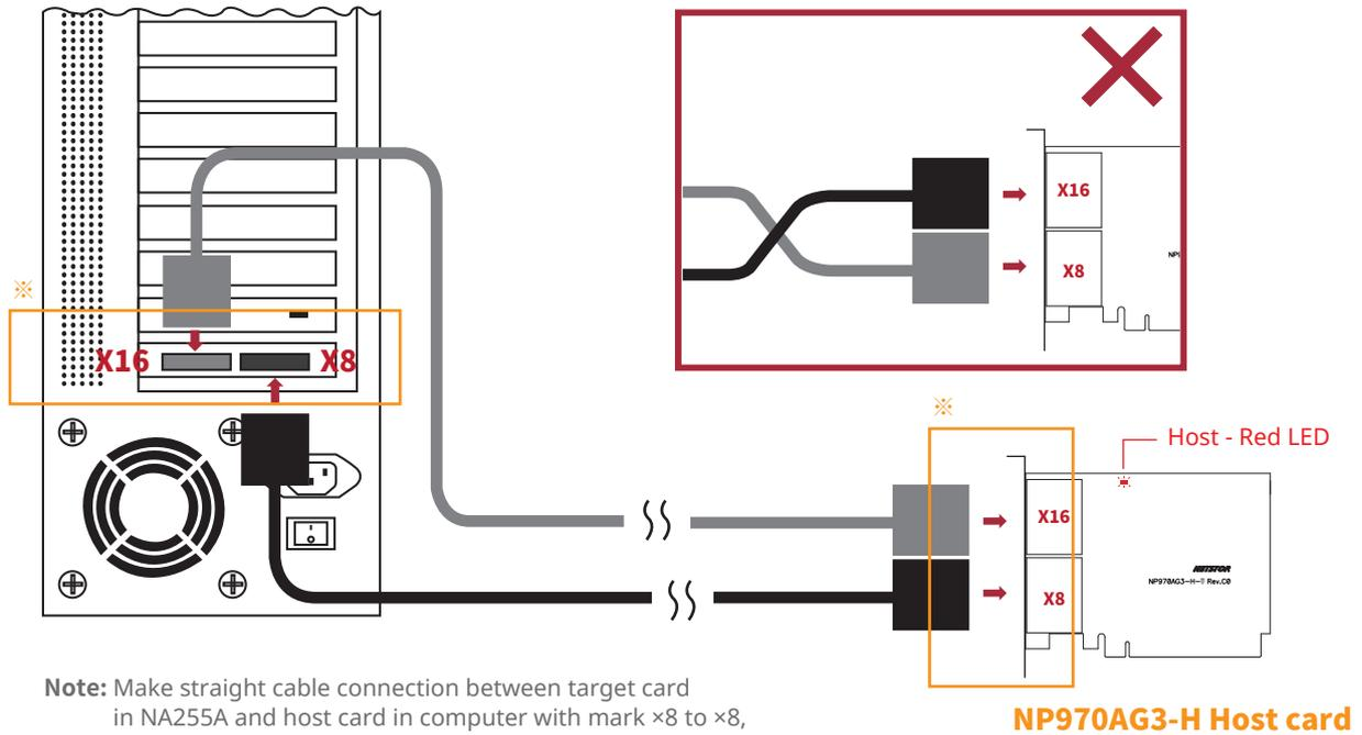
※ Note the ring-pull of the external PCIe x8 data cable connector must be at the same side as Netstor host card and target card's obverse side when cable is connected to the host/target card.
