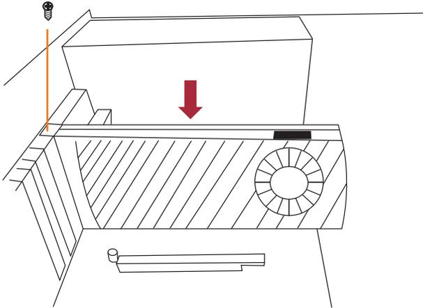
5. Each graphics card in NA255A is provided with supplementary 6+2 pin and 6-pin PCIe power cables for sufficient power. Up to four dual-width, full-length graphics cards can be installed in slots 2 ~ 5 in the Netstor chassis.
