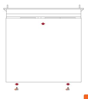
5. Connect the chassis and the host computer with external PCIe ×8 data cable. And
