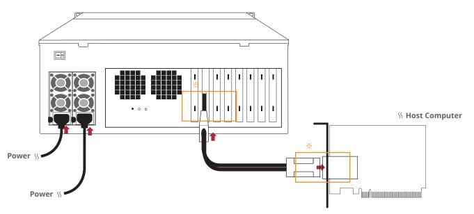
Note the ring-pull of the external PCIe ×8 data cable connector must be at the same side as Netstor host card and target card's obverse side when cable is connected to the host/target card.
