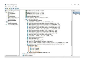
3. There will be PCI Express Root Ports with different ending numbers like 1C10, 1C18, and 1C1A. These different ending numbers indicate the different PCIe slots on computer motherboard.
