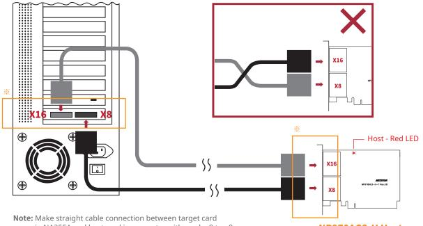
Ite: Make straight cable connection between target card in NA255A and host card in computer with mark ×8 to ×8, and ×16 to ×16. Do NOT make cross cable connection.
