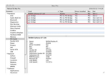
4. As graphics/PCIe cards are installed in NA255A, the graphics/PCIe cards will appear below the four pci-bridges.
