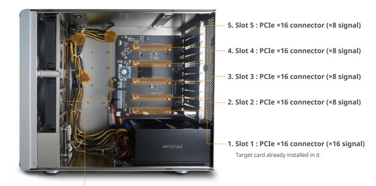
6. 4×6+2 pin PCIe power cables & 4×6-pin PCIe power cables for cards
