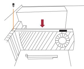
5. Each graphics card in NA255A is provided with supplementary 6+2 pin and 6-pin PCIe power cables for sufficient power. Up to four dual-width, full-length graphics cards can be installed in slots 2 ~ 5 in the Netstor chassis.
