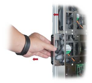
2. The front 120×120×25 mm cooling fan speed can be adjusted. Pull out the fan module, there are four sets of jumpers labeled with 6V, 8V, 10V, 12V from top to bottom on the fan connector board. The default setting is the jumper being placed over pin 7 and 8 for label 6V for slowest speed. The speed increases from label 8V to label 12V. As jumper is not placed over pins, the fan will spin at 12V full speed.
