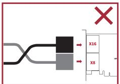
\*\* Note the ring-pull of the external PCIe ×8 data cable connector must be at the same side as Netstor host card and target card's obverse side when cable is connected to the host/target card.
