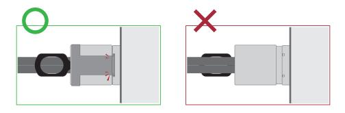
8. Connect one end of power cord to NA265A's power receptacle and the other end of power cord to grounded outlet or power strip.
