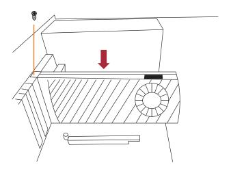
5. Each graphics card in NA265A is provided with two supplementary 6+2 pin PCIe power cables for sufficient power. Up to four dual-width, full-length graphics cards can be installed in slots  $2 \sim 5$  in the Netstor chassis.
