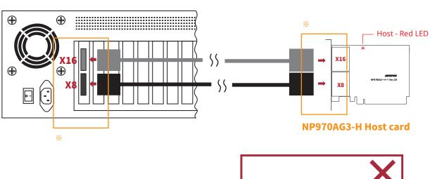
Note: Make straight cable connection between target card in NA265A and host card in computer with mark ×8 to ×8, and ×16 to ×16. Do NOT make cross cable connection.
