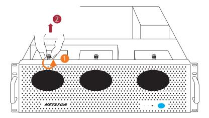
2. The front 90×90×25 mm cooling fan speed can be adjusted. Pull out the fan module, there are four sets of jumpers labeled with 6V, 8V, 10V, 12V from top to bottom on the fan connector board. The default setting is the jumper being placed over pin 7 and 8 for label 6V for slowest speed. The speed increases from label 8V to label 12V. As jumper is not placed over pins, the fan will spin at 12V full speed.
