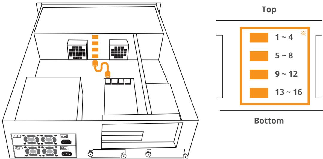
※ Note: when inserting the mini-SAS cable to the SFF-8087 port on drive backplane, the metal hook on the SFF-8087 connector on data cable must be facing upward.
