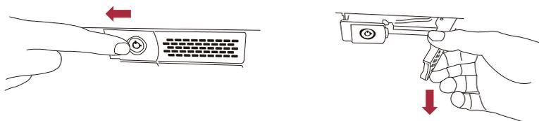
7. Place hard drives in the trays and fix them with hard drive mounting screws. Insert HDD trays back to NA333A-G3 storage enclosure.
