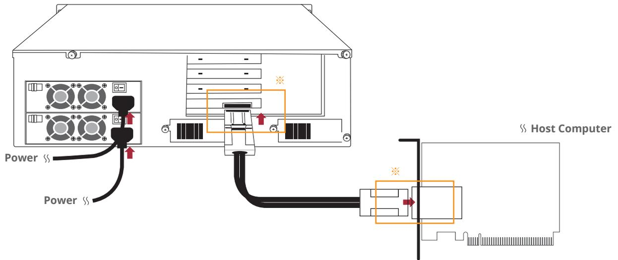
※ Note the ring-pull of the external PCIe ×8 data cable connector must be at the same side as Netstor host card and target card's obverse side when cable is connected to the host/target card.
