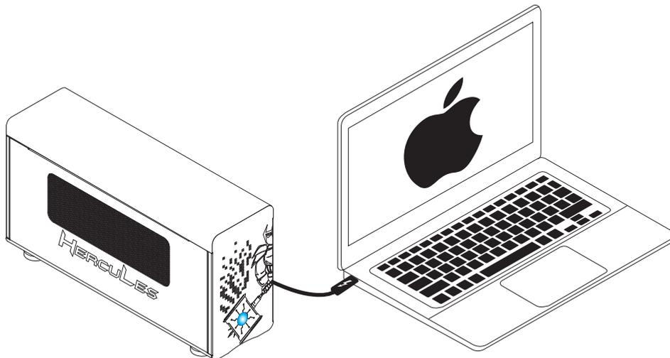
2. The HL23T-PRO enclosure is designed to be powered on/off simultaneously with Thunderbolt host computer when Netstor unit is connected to computer by Thunderbolt cable. Therefore, power on computer first, and then Netstor unit will be powered on automatically.
