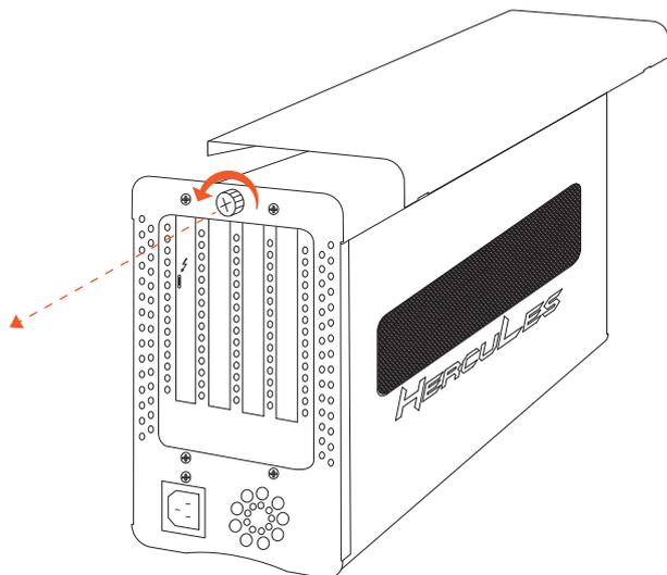
2. The PCIe slot at rear panel of HL23T-PRO is pre-covered by two removable L-shape metal brackets. Loosen the screws of the removable L-shape metal brackets for graphics card installation.
