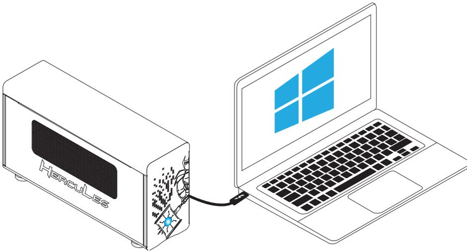
2. The HL23T-PRO is designed to be powered on/off simultaneously with Thunderbolt host computer as Netstor unit is connected to computer by Thunderbolt cable. Thus power on computer first, and then Netstor unit will be powered on automatically.
