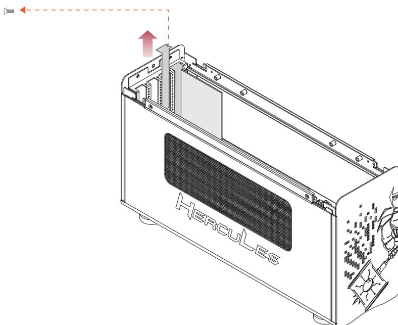
3. Install graphics card in the PCIe slot within the enclosure and tighten it with screw on graphics card's bracket.
