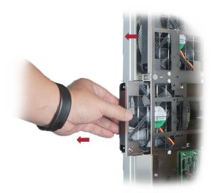
2. The front 12×12 cm cooling fan speed can be adjusted. Pull out the fan module; there will be three sets of pins marked with 8V, 10V, and 12V from top to bottom on the fan connector board. The default setting is the jumper being placed over pin 3 and pin 4 for 10V as the most-balanced medium speed. Additionally, according to the application situation, user can set it to 12V for highest speed, or set it to 8V for lower speed.
