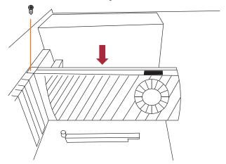
5. Graphics cards in NA255A-G4 are provided with supplementary 12+4-pin (16-pin) 12VHPWR power cables from Netstor unit's PSU for sufficient power. Up to four graphics cards are allowed to be installed in slots  $2 \sim 5$  within the Netstor chassis.
