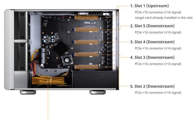
6. 12+4-pin (16-pin) 12VHPWR power cables for graphics cards
