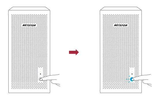
2. To disconnect NA255A-G4 from server, always power off server first, and then power off NA255A-G4. To power off NA255A-G4, press and hold the power LED button for over two seconds until LED button's blue light goes off.
