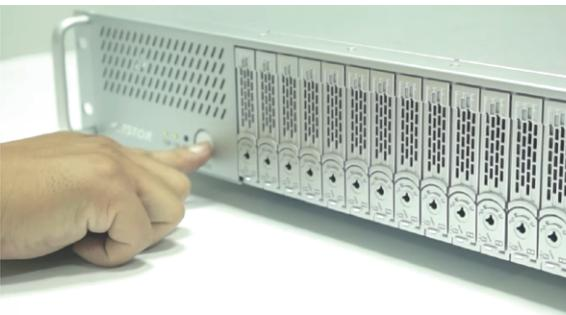
3. As the embedded Mac mini is connected to Netstor unit by Thunderbolt 3 cable, while shutting down Mac mini through macOS, the entire NA338TB3 system will be powered off simultaneously.
