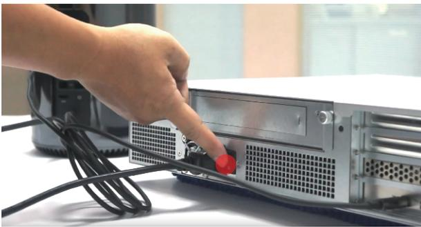
2. The NA338TB3 is designed to be powered on/off simultaneously with the Thunderbolt 3 host computer, so when computer is connected to Netstor unit externally by Thunderbolt 3 cable, power on the host computer first, and then NA338TB3 will be powered on automatically. (NA338TB3 also supports hot-plug and hot-unplug for powering on and off)
