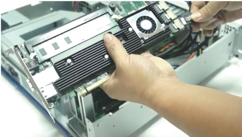
7. Install RAID card and other third-party PCIe cards into the proper PCIe slots within NA338TB3 and tighten them with screws on third-party PCIe cards' brackets.
