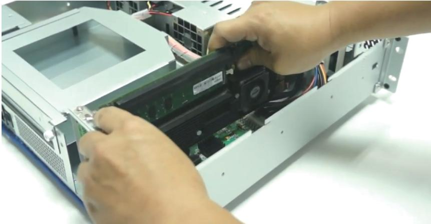
8. When RAID card and the other third-party PCIe cards are installed properly, restore the PCIe expansion unit from upright position to the original horizontal position. And screw the four black screws back to the unit.
