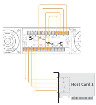
2×2 backplane & 1×4 backplane NS388P enclosure and host card connection diagram.
