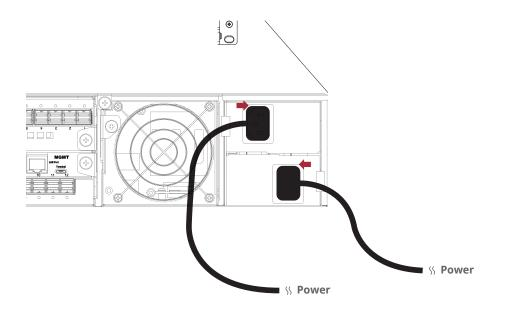
9. After the two power cords are connected properly, you can then press the power button for over two seconds at rear of NS388P to power on the Netstor unit, and then power on the server/workstation.
