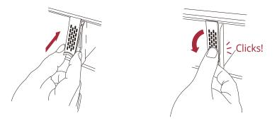
※ Do not force the levers to close while you insert U.2 drive modules into the enclosure. If a lever does not close smoothly, draw out and insert the U.2 drive module again, and then press the lever to close.
